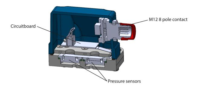
In order to get the unit to work properly with good accuracy, it is very important that the unit is installed correctly according to the installation instruction, see chapter **10.5 Installation and changing of Control unit.**
