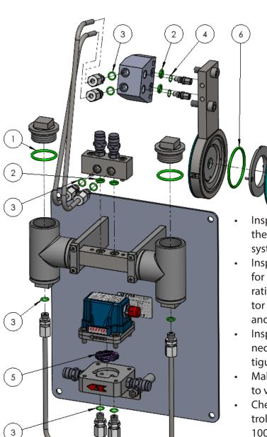
Inspect the orifice plate on a regular basis. Check for damage, dirt build-up and that the edge of the orifice plate is still sharp. The sharp edge of the bore is crucial to provide proper and accurate flow reading. If the bore wear is excessive, please contact a local distributor or Eletta Flow for purchase of a replacement orifice.
